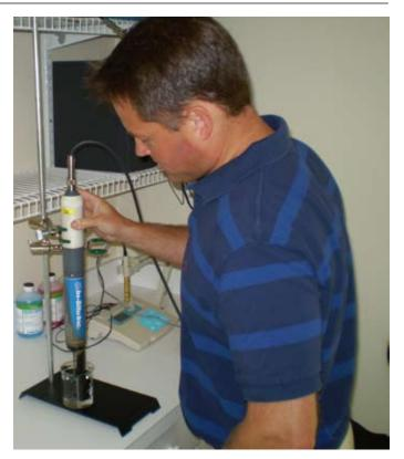
Figure 4: Mike Piehler calibrates the TROLL® 9500 Water Quality Instrument in the laboratory before deploying it to an outfall monitoring site.
