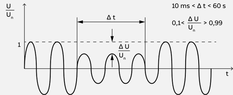
Schematic representation of a voltage dip.
